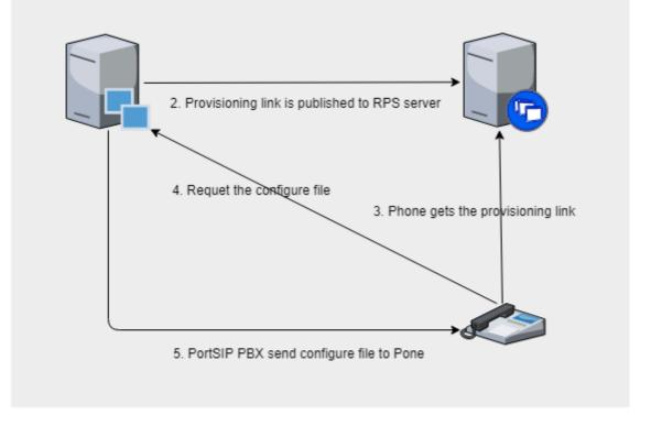
In the case PortSIP PBX locates in cloud, IP Phones can be auto provisioned via RPS (RPS is a service provided by IP Phone vendors). PortSIP PBX supports for Yealink, Htek, and Fanvil RPS. If you are using the IP Phone from one of the providers above, you may configure your IP Phone in a very easy way, without the need to manually copy the auto provisioning link (in this scenario the PnP mode is unavailable).
