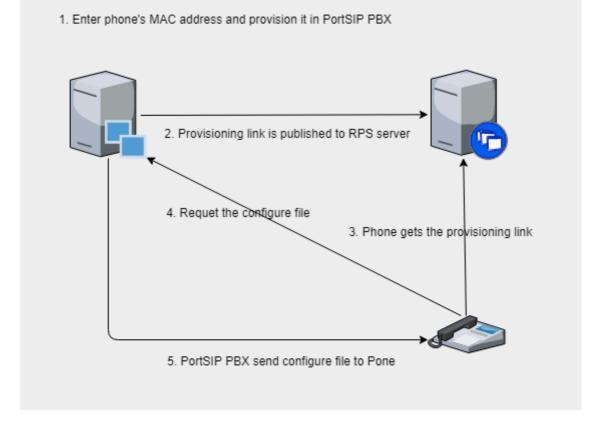
In the case PortSIP PBX locates in cloud, IP Phones can be auto provisioned via RPS (RPS is a service provided by IP Phone vendors). PortSIP PBX supports for Yealink, Htek, and Fanvil RPS. If you are using the IP Phone from one of the providers above, you may configure your IP Phone in a very easy way, without the need to manually copy the auto provisioning link (in this scenario the PnP mode is unavailable).
