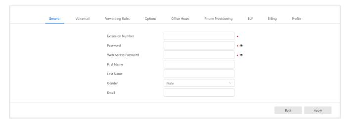
To configure an extension, click on "Call Manager > Extensions" in the PortSIP PBX Web Portal. Click on "Add" to create a new one, or select an existing extension and click the Edit button to configure or manage the existing extension users. "Web Access Password" is used by extension users to log into Web Portal.
