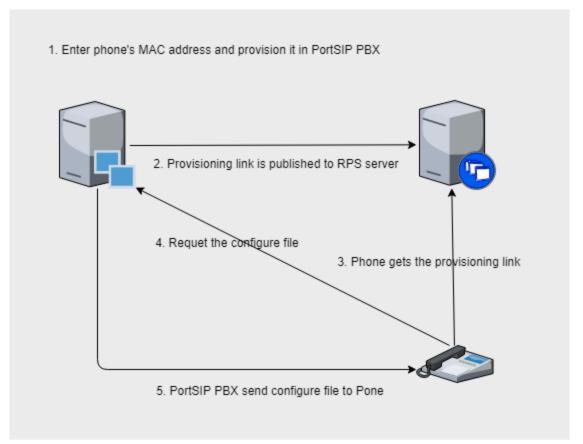
In the case PortSIP PBX locates in cloud, IP Phones can be auto provisioned via RPS (RPS is a service provided by IP Phone vendors). PortSIP PBX supports for Yealink, Htek, and Fanvil RPS. If you are using the IP Phone from one of the providers above, you may configure your IP Phone in a very easy way, without the need to manually copy the auto provisioning link (in this scenario the PnP mode is unavailable).
