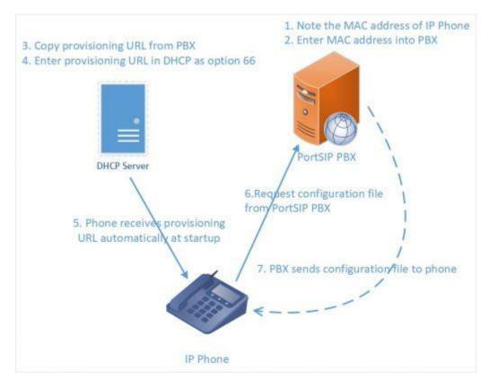
Cisco, Polycom and Aastra phones do not support plug and play nor secure HTTPS provisioning with a Let's encrypt Root CA or self-signed CA. They can only be used on the local LAN and must be provisioned as follows:
